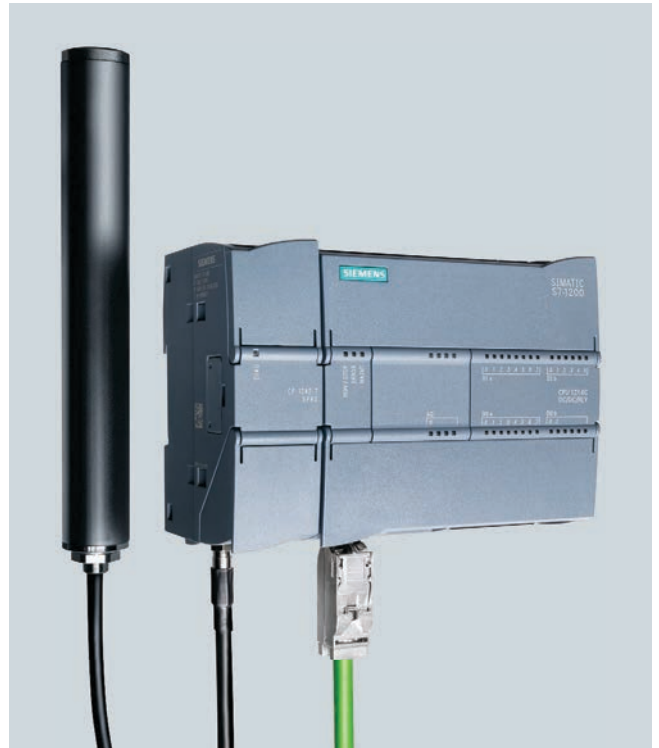
The two RTUs (Remote Terminal Units) in Nicaragua each consist of a SIMATIC S7-1200 controller with CP 1242-7 communication processor. The values measured on site are directly transmitted to the "control center" at the school in Hamburg via GPRS.
